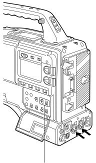
Up to two external microphones can be connected to the AUDIO IN CH1/CH2 Connectors.
